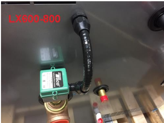
Fig. 4 Final Paddle Assembly
