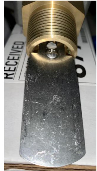
Fig. 3 Final Paddle Assembly
