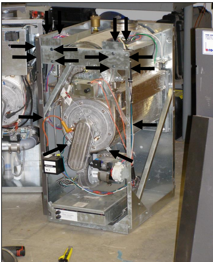
Figure 6: Lx300-399 hold down brackets
